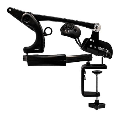
Syrebo® Dynamic Arm Support is an upper limbassisted rehabilitation robot developed specifically for users with limited upper limb function caused by neurological disorders such as stroke, traumatic brain injury, and spinal cord injury.
