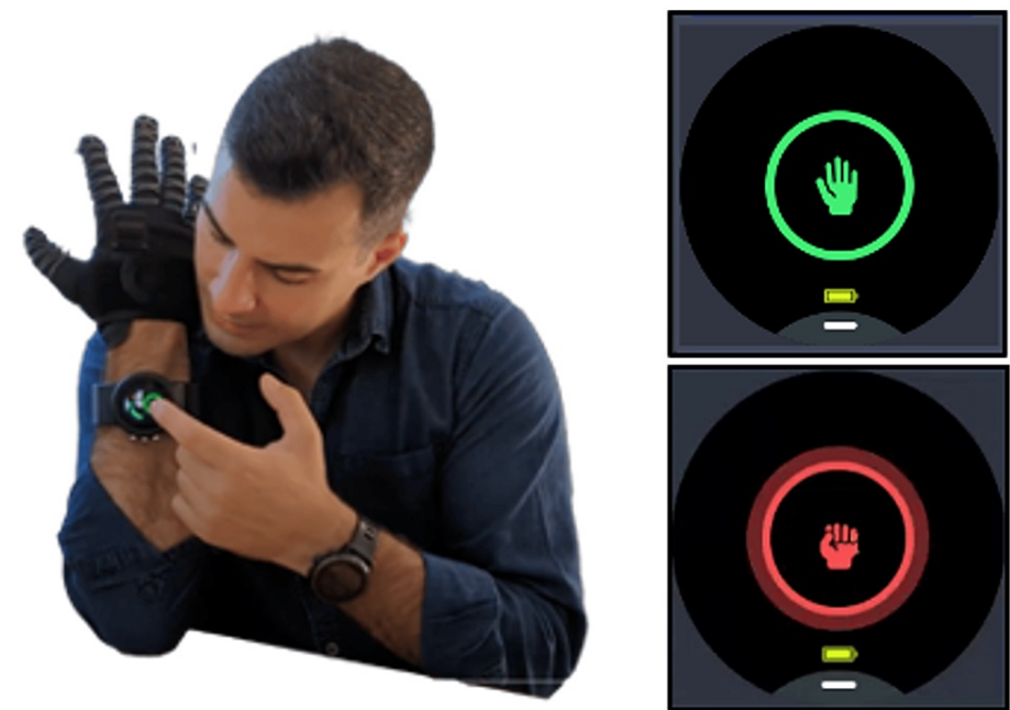
FIGURE 2: Toggling locking states of the Nuada Glove. Clicking the touchscreen (left) toggles the states (right) between inactive (up) and active (down).
